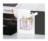
We have integrated a manual oiler into the device which will ensure it runs smoothly, giving a consistently high cutting capacity and quality.
