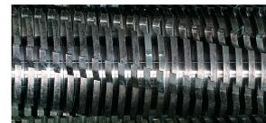
The induction-hardened, solid steel cutting rollers are robust and ensure a high level of durability.
